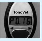
Press the measurement button to exit the old values search. Old is on the display. Press either of the selector buttons to access the other functions (00=measurement, End=turning OFF).
