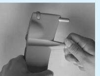
Screw the collar in, to lock the probe base.
