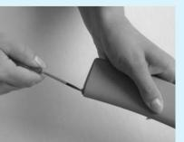
Put new AA batteries into the tonometer according to figures inside the battery compartment. +terminals should be down on the display side of the tonometer (behind). -terminals should be up on the measurement side (the front side).
